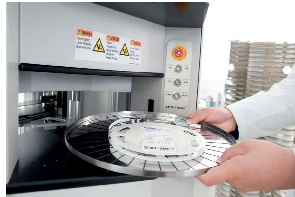
→ Preloaded Agilis feeder stored in SMD Tower.
