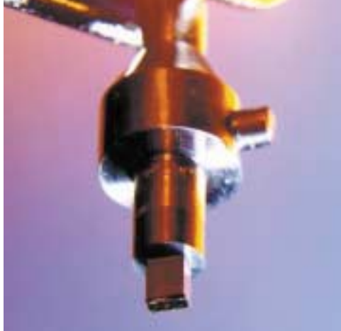
Figure 3. Inverted pyramid collet for eutectic bonding.
