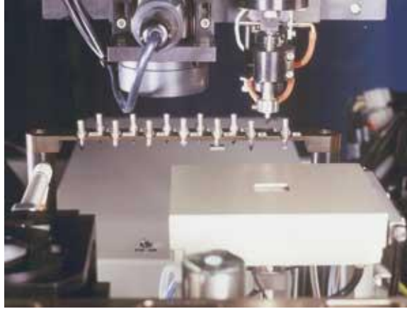
Figure 1. Automatic tool changing provides capability for handling the widest range of components and die.
