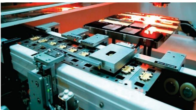
**Figure 2:** “Universal” progress indexing conveyor.
